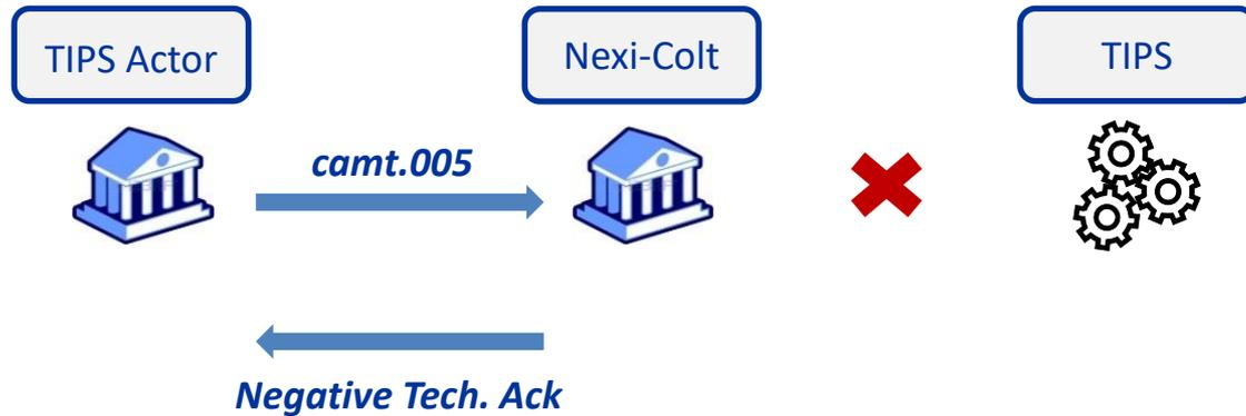
Nexi-Colt directly rejects the XML message via Technical Ack negative response (SendErr)
